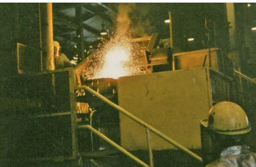
Smaller scale water atomisers are used in precious metal applications, including dental amalgam production. Large scale water atomisers can be seen making Fe powder for PM applications or atomising alloys for further refining, such as the FeCoCuS Matte atomiser in Chambishi, Zambia. Atomising Systems Ltd. has supplied systems to suit such client requirements.
